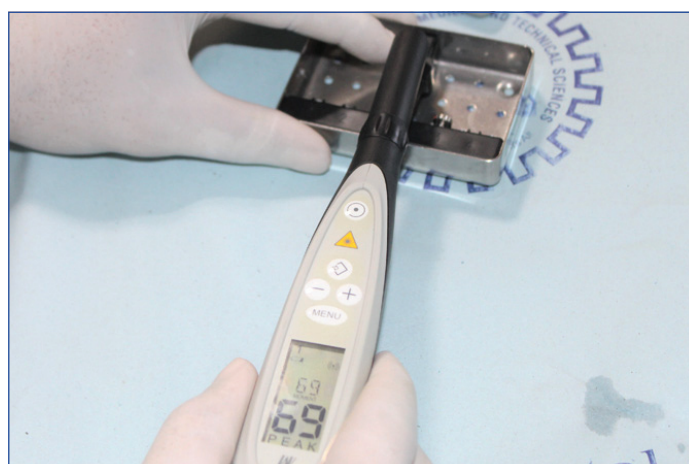
[Table/Fig-2]: Calibration value in the display agrees with the reference value at 90° angle. Reference value is engraved on the surface of the calibration disk.
