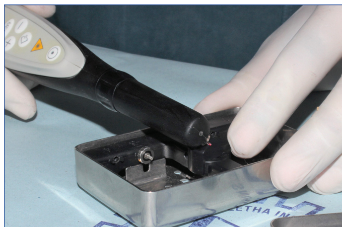
[Table/Fig-1]: Calibrating the Diagnodent (DD) with the selection of probe tip to achieve specific zero baseline.
